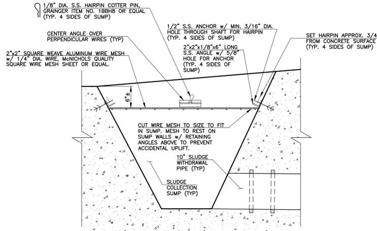
**1 SECONDARY CLARIFIER SLUDGE SUMP SCREEN SECTION**
