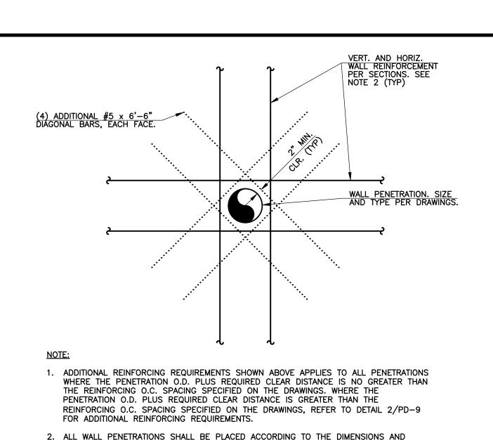
2. ALL WALL PENETRATIONS SHALL BE PLACED ACCORDING TO THE DIMENSIONS AND ELEVATIONS SHOWN ON THE DRAWINGS. WHERE THE WALL PENETRATION DOES NOT FALL BETWEEN REINFORCING BARS, PROVIDE (1) VERTICAL AND HORIZONTAL REINFORCING BAR ON EACH SIDE OF THE PENETRATION AT THE CLEAR DISTANCE REQUIRED. THEN RESTART THE REINFORCING O.C. SPACING SPECIFIED ON THE DRAWINGS TO THE OPPOSITE SIDE OF THE PENETRATION. DO NOT EXCEED THE REINFORCING O.C. SPACING SPECIFIED ON THE DRAWINGS.
