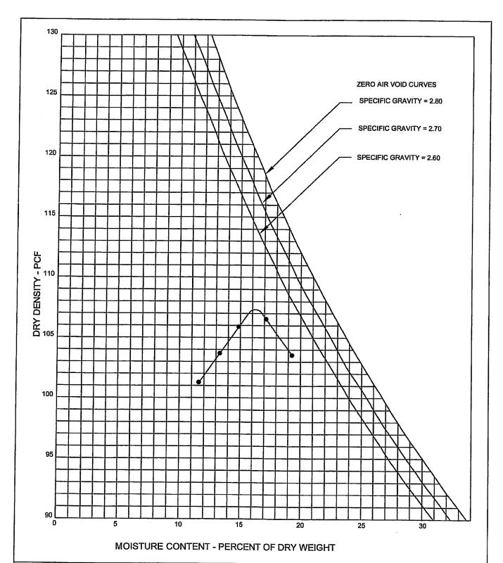
LOCATION: HDT REGIONAL WATER RECLAMATION FACILITY MOISTURE-DENSITY **RELATIONSHIPS** B3 @ 1-3 feet SOIL DESCRIPTION: Sandy clay (CL) HEPWORTH-PAWLAK GEOTECHNICAL, Inc. MAX. DRY DENSITY: 107.3 OPT. MOIST. CONTENT: 16.2 % PROCEDURE: ASTM D698 LIQUID LIMIT: 35 PLASTICITY INDEX: 19 JOB NO.: 308121B GRAVEL: % SILT AND CLAY (-200): 72 % % SAND: DATE: 1-29-08 Fig. 20
