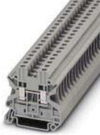
Feed-through terminal block, Connection method: Screw connection, Cross section: 0.14 mm 2 - 6 mm 2 , AWG 26 - 10, Width: 6.2 mm, Color: gray, Mounting type: NS 35/7.5, NS 35/15
